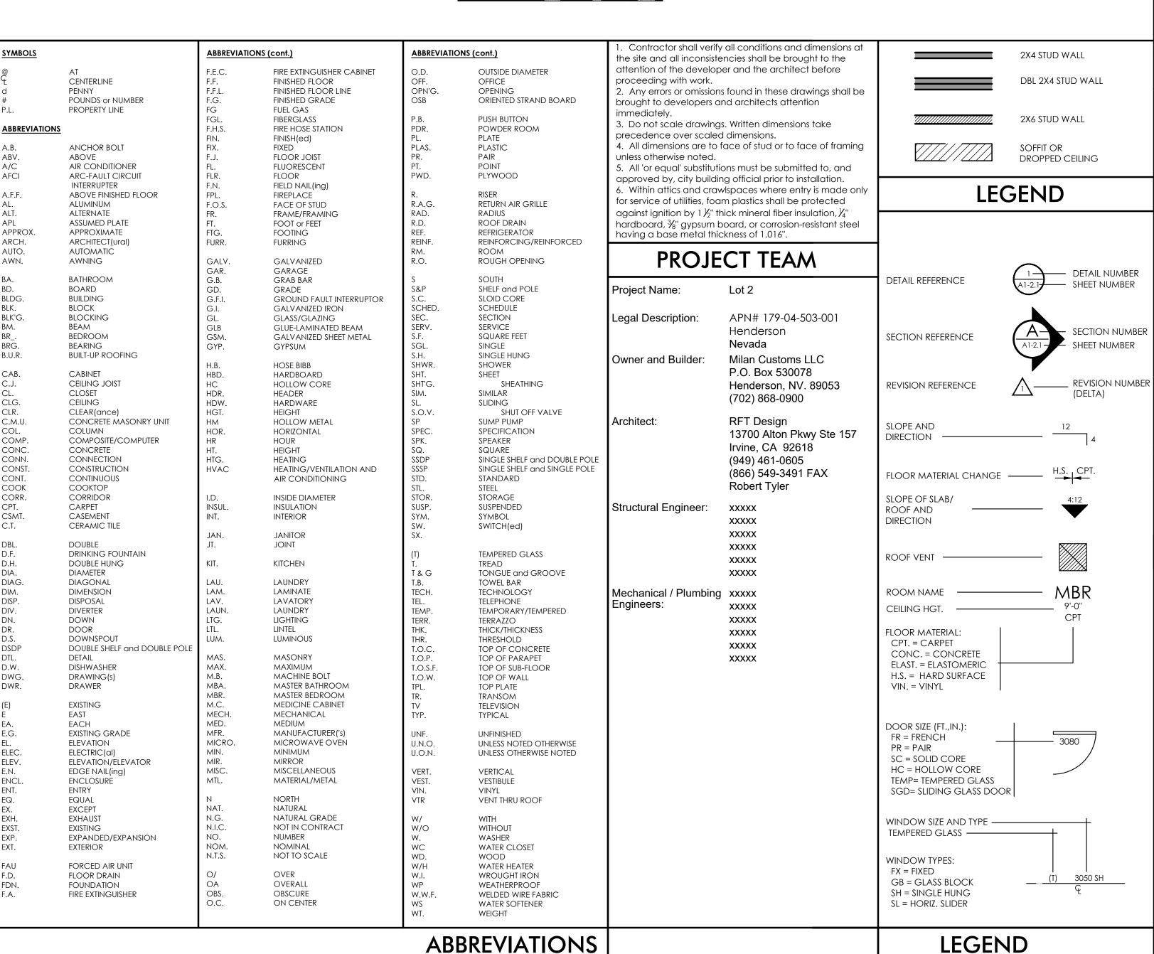
WRITTEN DIMENSIONS TAKE PRECEDENCE OVER 8. CLOTHES DRYER EXHAUST: SCALED DIMENSIONS. DO NOT SCALE DRAWINGS. REFER TO ENERGY COMPLIANCE INFORMATION FOR HVAC EFFICIENCY, GLAZING U-VALUES, SHADING DEVICES AND INSULATION VALUES. SAFETY GLAZING SHALL BE PROVIDED IN THE FOLLOWING LOCATIONS: i. INGRESS AND EGRESS DOORS, FIXED AND
